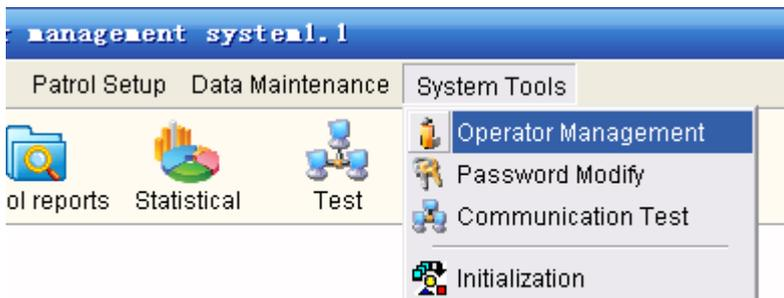
b. Press **System Tool**, and choose **Operator Management**, and then click on **Modify** to reset username and password at different access level. Customers can click **Add** to add new username and password.
